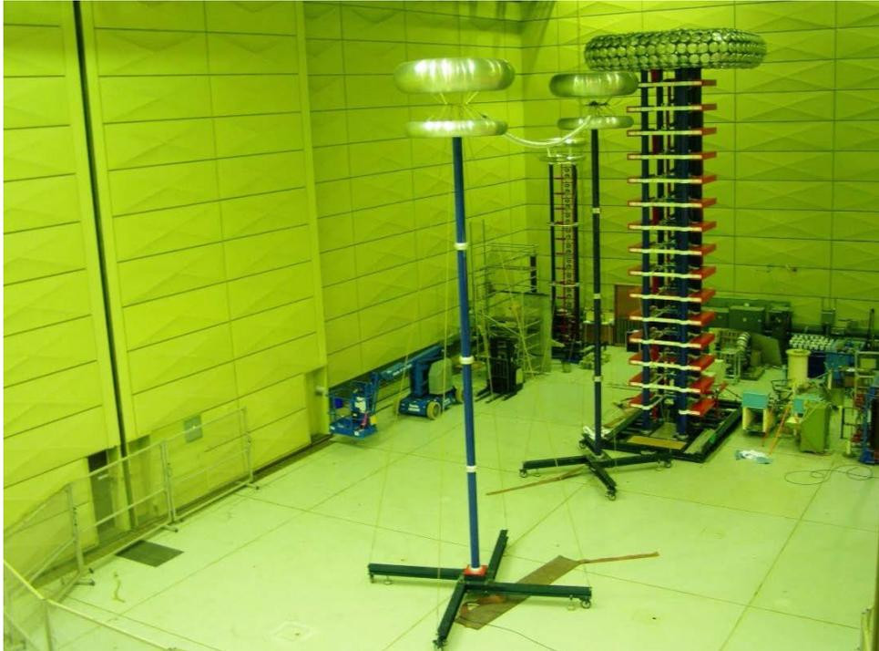
Figure 2 The 2800 kV voltage divider for measuring steep impulse voltages
